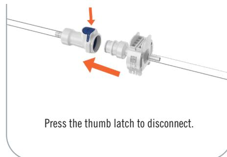
Press the thumb latch to disconnect.
